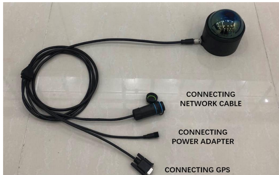
Figure 3.1 Connecting Lidar and Computer
